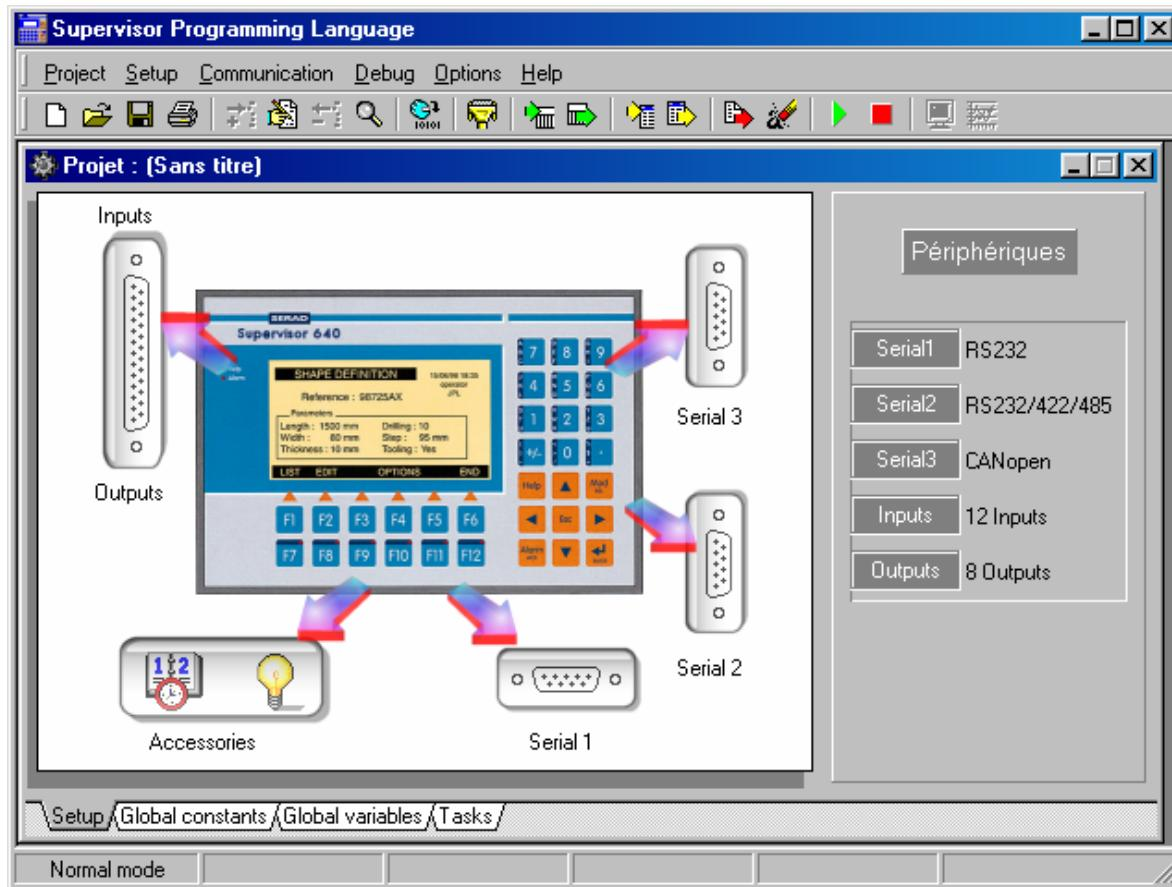
On the configuration window, there are two zones. The first zone is on the left with the front of SUPERVISOR. This zone allows the SUPERVISOR configuration. We can configure the display machine, the SERIAL1, SERIAL2, SERIAL3, INPUTS and OUTPUTS. The second zone is on the right with the name « Périphériques » give the affectation of the different connectors.
