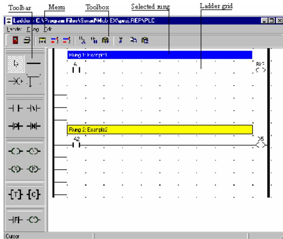
The ladder editor is composed with an editor zone of the ladder program (the grid), a toolbar of chart that can be inserted and a toolbox. A ladder program have lot of rungs limited to 50 in a task. Each rungs have an optional comment, an expression and 1 to 5 outputs.
